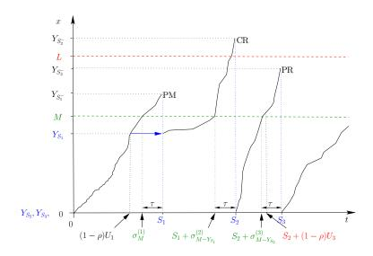
FIGURE 1: The condition-based maintenance policy
