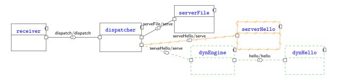
Figure 3: The software architecture of the web server after dynamic reconfiguration.
