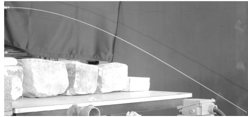
Figure 5: Aluminium bar bending under its own weight.
