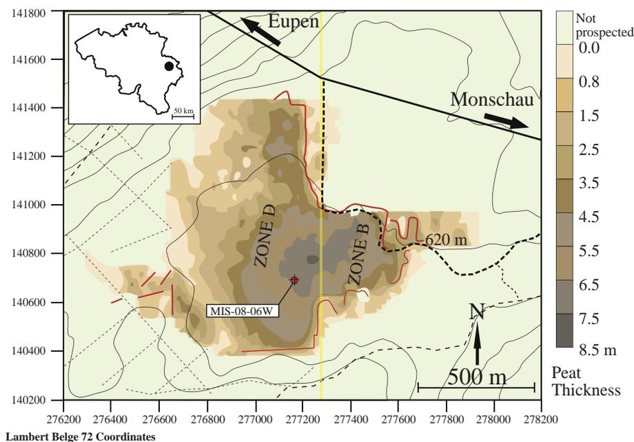
**Fig. 1.** The Misten bog (south of the Eupen-Monschau road) and the location of the MIS-08-06W peat profile. Peat thickness after Wastiaux and Schumacker (2003). Dotted lines are access pathways. Red lines are the cutting fronts (stopped during the 2nd world war). The yellow stripe represents the main drain, dug in 1774 and active until 1970). (For interpretation of the references to colour in this figure legend, the reader is referred to the web version of this article.)
