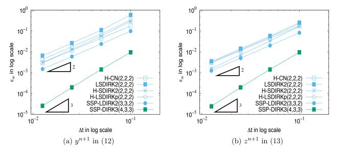
FIGURE 3. Test 1 - Reaction-diffusion problem:  $L^{\infty}$  error norm when the last step is performed using the coefficients obtained from the (a) explicit scheme (12) and (b) and the implicit scheme (13) for the IMEX schemes described in the previous section.
