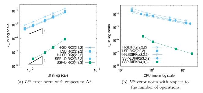
FIGURE 5. Test 2 - Nonlinear convection-diffusion problem: (a)  $L^{\infty}$  error norm for the second order schemes (22), (25), (23), (24) and (26) and the third order SSP-DIRK3(4,3,3) L-stable scheme (27).
