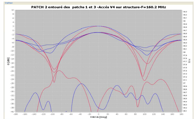
Figure 10: Measured radiation pattern of the central element in the array (port 4: V-polarization perpendicular to the array axis)
