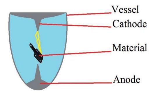
Figure 7 Schematic view of the high-voltage fragmentation process
