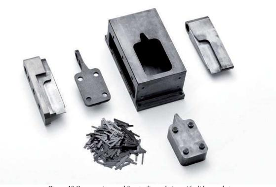
$Figure\ 10\ Compression\ moulding\ tooling\ solution\ with\ sliders\ and\ stamp$
