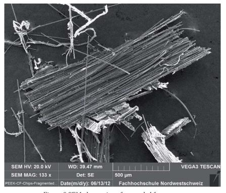
Figure 8 SEM observation of a recycled fragment
