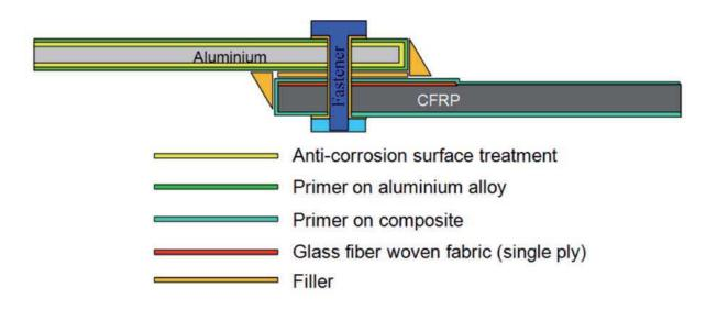
Figure 1 EASA recommended protection against galvanic corrosion
