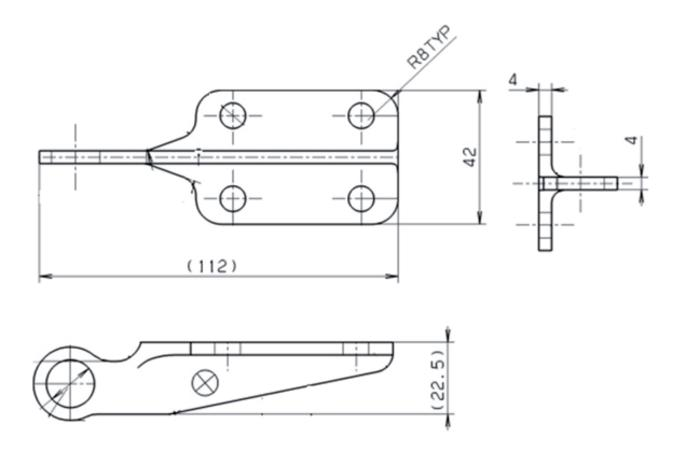
Figure 3 Dimensions of the CNC-machined steel door hinge (courtesy of Eurocopter Germany GmbH)
