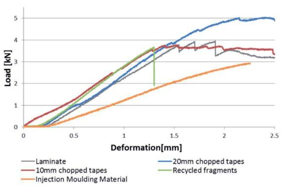
Figure 12 Representative load-deformation curves for each material type
