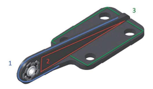
Figure 11 Zone definition for the laminate-based door hinges
