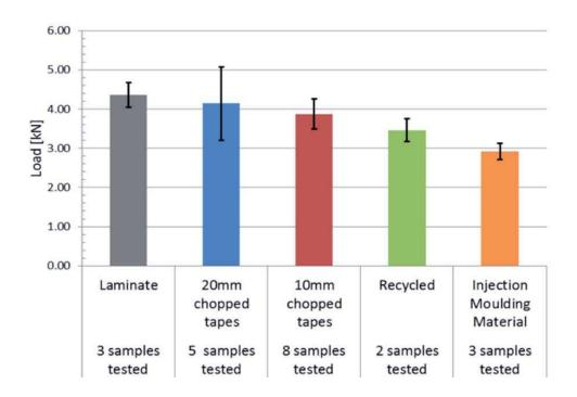
Figure 13 Ultimate load measured for each type of material
