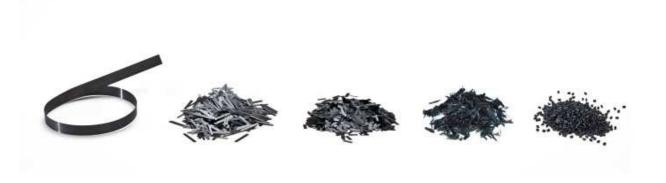
Figure 6 From left to right, UD tape, 20mm chopped tapes, 10mm chopped tapes, recycled fragments, injection moulding granules
