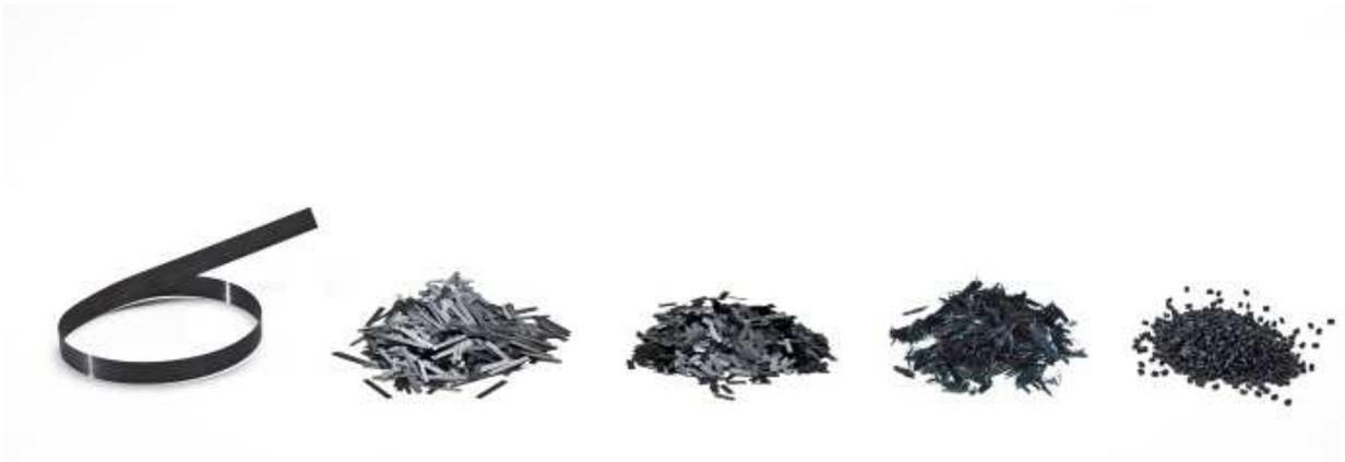
Figure 6 From left to right, UD tape, 20mm chopped tapes, 10mm chopped tapes, recycled fragments, injection moulding granules
