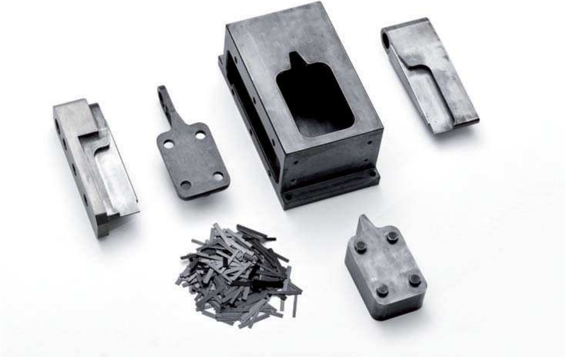
Figure 10 Compression moulding tooling solution with sliders and stamp
