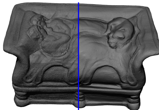
Figure 1: The Lovers of Bordeaux (15.8 million points). Exploiting self-similarity in the model, we compress this representation down to 1.15 MB. The resulting model (right) is very close to the original one (left), as the reconstruction error is less than the laser scanner precision (0.02mm) for 99.14% of the input points.
