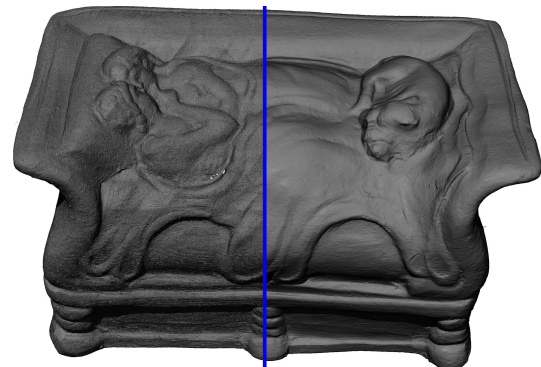
Figure 1: The Lovers of Bordeaux (15.8 million points). Exploiting self-similarity in the model, we compress this representation down to 1.15 MB. The resulting model (right) is very close to the original one (left), as the reconstruction error is less than the laser scanner precision (0.02mm) for 99.14% of the input points.
