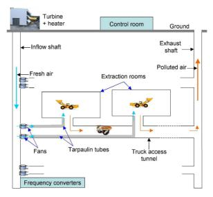
Fig. 1 Airflows in an underground mine.
