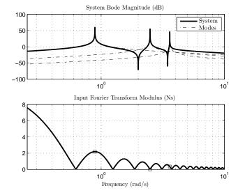
Figure 2. Bode diagram and input Fourier transform: case 1 (rectangular input).
