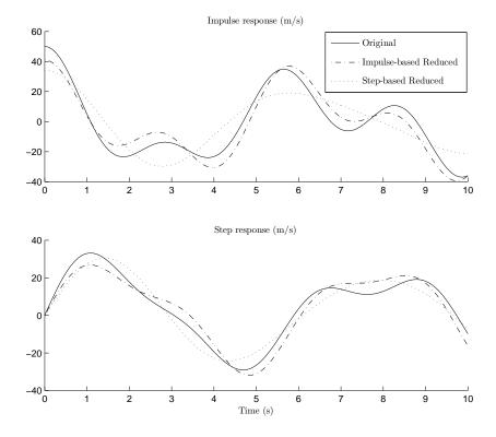
$Figure \ 6. \ \textit{Impulse and Step responses of the original system, impulse-based reduction system and } \\$  $step\text{-}based\ reduction\ system.$
