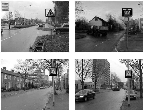
Fig. 14 Detection Results: warning and yield traffic signs
