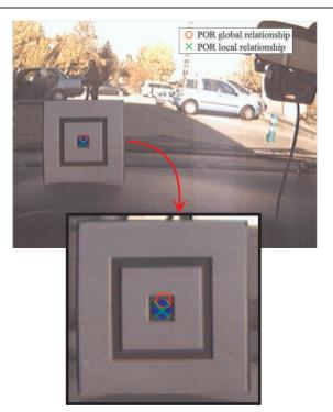
Fig. 14 Experimental results through a calibration with a single point. Local method: green and global method: in red. The distance between the two solutions is 7 pixels.
