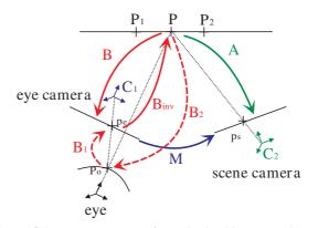
Fig. 5 Schematic top view of standard calibration. The projection of point P in the scene camera is  $p_s$  and the projection of the pupil centre looking at point P is  $p_e$  on the eye camera. P,  $P_1$  and  $P_2$ : points on the pattern.
