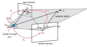
Fig. 15 Model of the ET system and the eye. Point P is in the same projection on the eye and the eye camera anywhere on line D. But the projections from point P in the scene camera are not merged, the projections form an epipolar line  $D_s$
