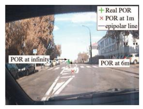
Fig. 21 The POR estimated at 1 metre is substitued by a segment of the epipolar line. The segment starts for Z = 6m and ends for  $Z \to \infty$ . This segment mesure approximately 15 pixels.
