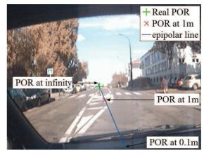
Fig. 20 The driver looks at a road sign. The ET system is calibrated at 1m and the object viewed is at 10m approximatively. By measuring  $T_x$ ,  $T_y$  and  $T_z$  it is possible to reduce the uncertainty range of the parallax phenomenon and thus draw an epipolar line.
