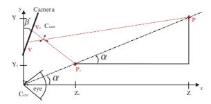
Fig. 16 Parallax between the eye and the scene camera. Points  $P_c$  and P are the same projection on the eye in two positions, but the projections of the point  $P_c$  and P in the scene camera are not merged.  $Z_c$  is the calibration distance.
