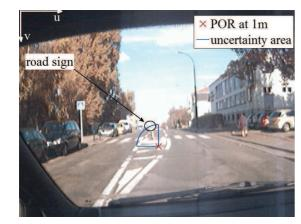
Fig. 19 The driver looks at a road sign. The ET system is calibrated at 1m and the object viewed is at 10m approximatively. The uncertainty range of the parallax phenomenon is the quarter of the blue disk.
