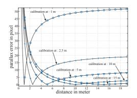
Fig. 17 Miscalculation of the POR due to the parallax phenomenon over a function of the distance.
