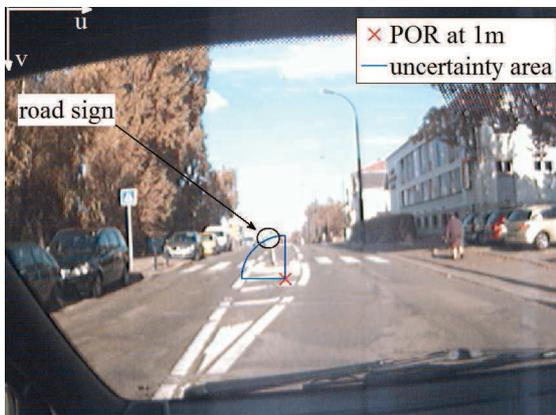
**Fig. 19** The driver looks at a road sign. The ET system is calibrated at 1m and the object viewed is at 10m approximately. The uncertainty range of the parallax phenomenon is the quarter of the blue disk.
