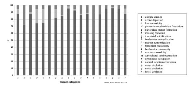
**Figure 1.** Environmental impacts due to the carbon reinforcement (*dark grey*), the epoxy matrix (*light grey*) and the injection moulding process (*intermediate grey*), while processing a 1 kg carbon/epoxy composite part. The analysis is based on Duflou *et al.* data [1].
