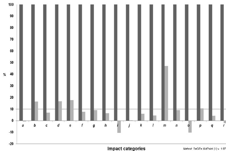
**Figure 3.** Comparison of the environmental impacts of a 1 kg composite part throughout its life cycle, and depending on the end-of-life option: dark grey refers to the landfill of the composite part, and light grey to reinforcement recycling (Caption: see above, figure 2)
