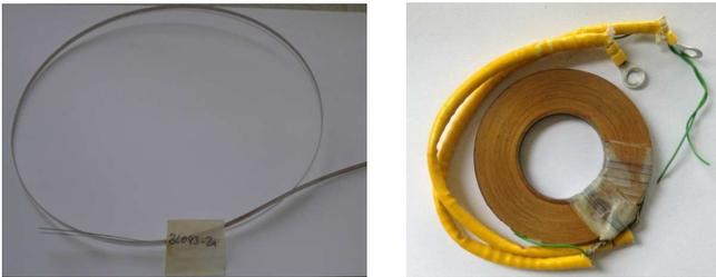
Fig. 10. Sample of superconducting wire (BSCCO2212) and superconducting coil used in the experiment (on the right side)
