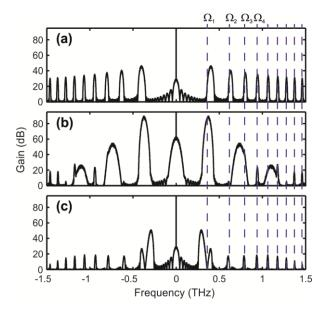
**Figure 1 :** Evolution of the output spectra recorded after 12 km of propagation for different values of the amplitude of the dispersion fluctuation:  $D_{amp} = 0.5$  ps/km/nm, 1.7 ps/km/nm and 3.7 ps/km/nm, subplots (a), (b) and (c) and respectively. The vertical dashed lines represent the predictions from Eq. (4).
