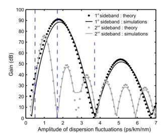
Figure 4: Evolution with  $D_{amp}$  of gain at the frequencies predicted by Eq. (0) for the first and second QPM sidebands (black and grey colors respectively). Results obtained from numerical simulations (solid lines) are compared with analytical predictions from Eq. (0) (circles and squares). Positions of the three cases reported in Fig. 1 are marked with dashed vertical lines.
