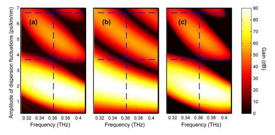
Figure 5: Magnification of the MI gain spectrum around the first QPM sideband vs.  $D_{amp}$ . Numerical results (a) are compared with the analytical results (b) predicted by Eq. (8) and by the Floquet linear stability analysis (c). Blue dashed vertical lines indicates the angular frequency  $\Omega_I$  as predicted from Eq. (0) and horizontal lines highlight the values of dispersion fluctuations that are then used in Fig. 6.
