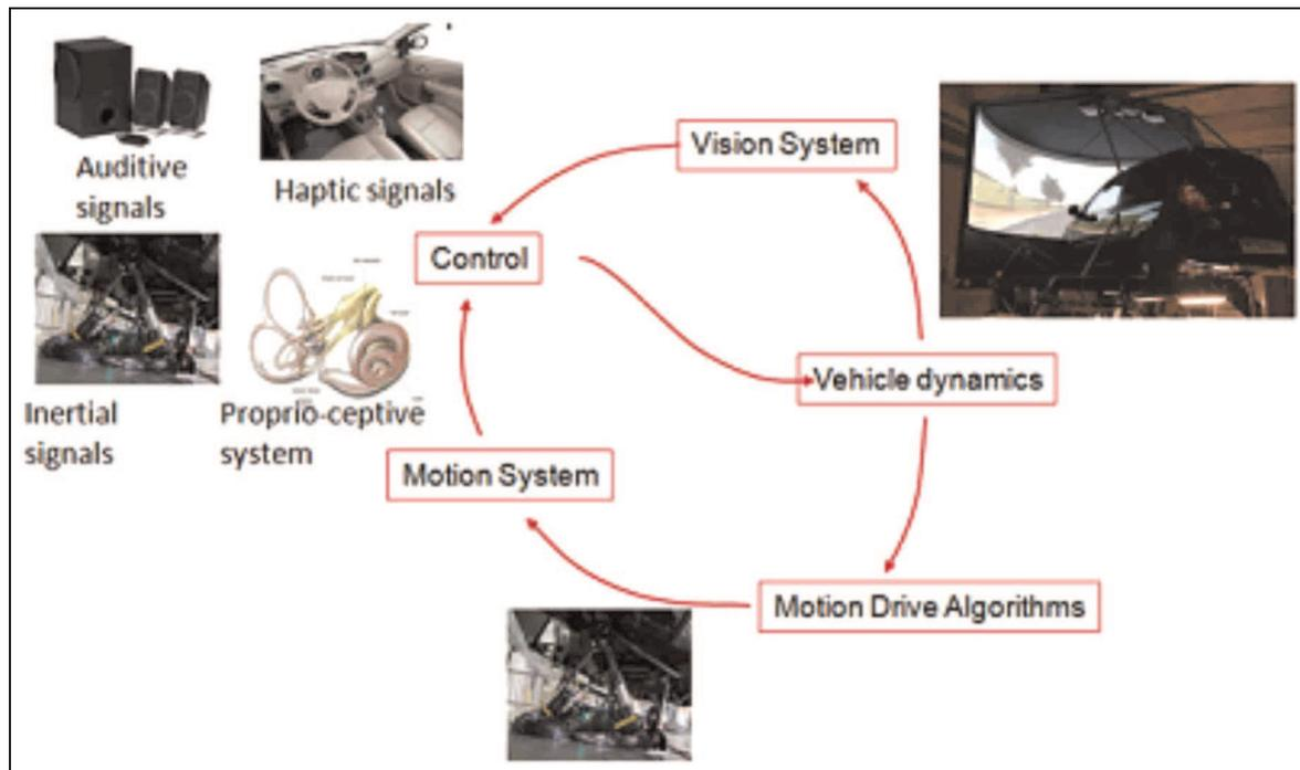
**Figure 1.** Structure of the closed-loop control of the dynamic driving simulator.<sup>8</sup>
