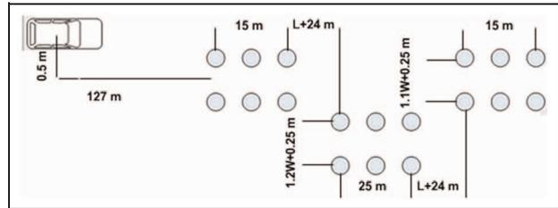
**Figure 4.** NATO chicane right turn used on the driving simulator session.<sup>31</sup>
