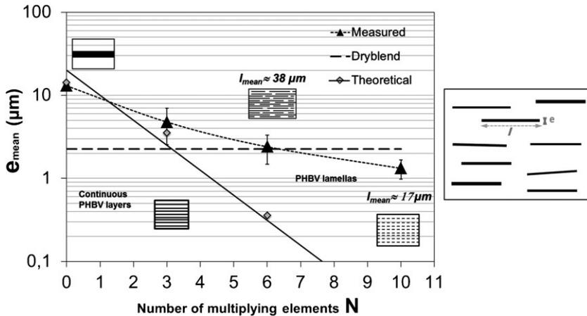
Figure 4. Comparing measured (for multilayer and dryblend films) and theoretical thickness of PHBV layers and lamellas (left). Schematic illustrating the dimensions of the lamellas (length  $l$ , thickness  $e$ ) (right). The mean values are calculated by measuring the dimensions for all the lamellas within a picture.
