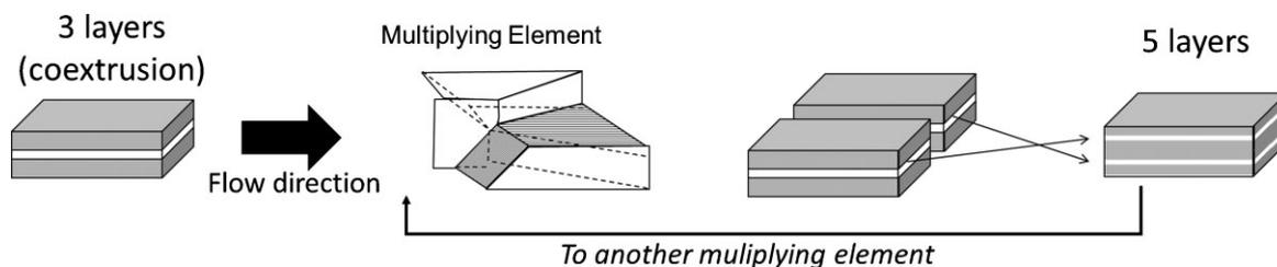
■ Figure 2. Schematic of the multilayer co-extrusion process.
