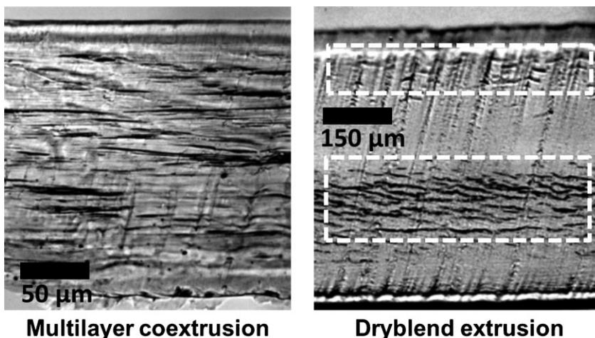
**Figure 8.** Dispersion of PHBV lamellas along film thickness for different films (six mixing elements on the left, dryblend on the right). Note that the dryblend presented here is thicker (same preparation method but no chill rolls), for illustration purpose.
