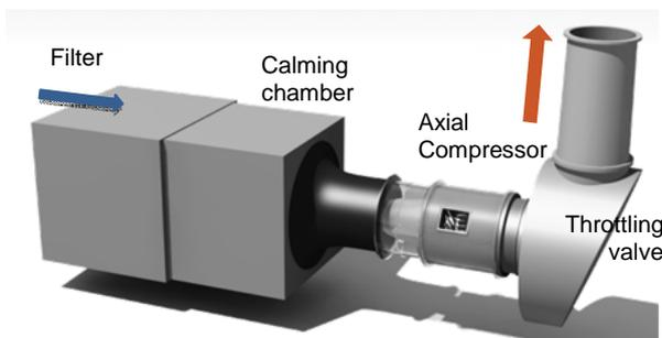
Figure 1 Compressor test rig
