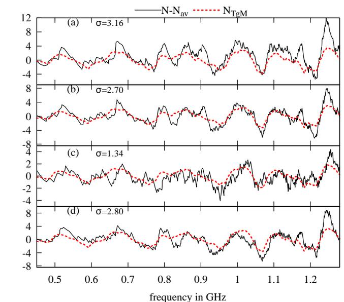
Fig. 14: Evolution of the spectral fluctuations. Fluctuating part of the counting functions,  $N-N_{av}$ , for (a) Cavity\_1, (b) Cavity\_2, (c) Cavity\_3 and (d) Cavity\_4 (continuous lines);  $N_{TgM}$  is the contribution of the tangential modes (red dotted line). The value of the standard deviation  $\sigma$  of  $N-N_{av}$  is indicated in the inset.
