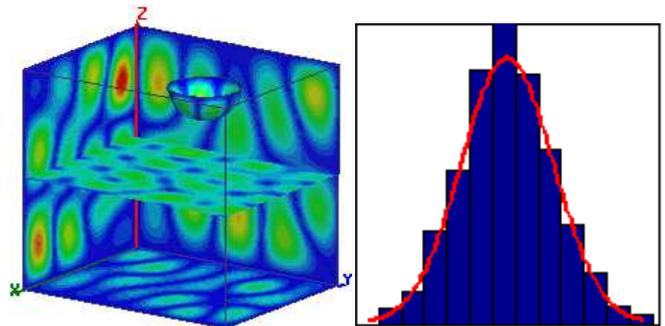
Fig. 3: Electric field amplitude and associated distribution of  $E_x$  component at 999MHz (232<sup>th</sup> mode) for Cavity\_1 (KS=0)
