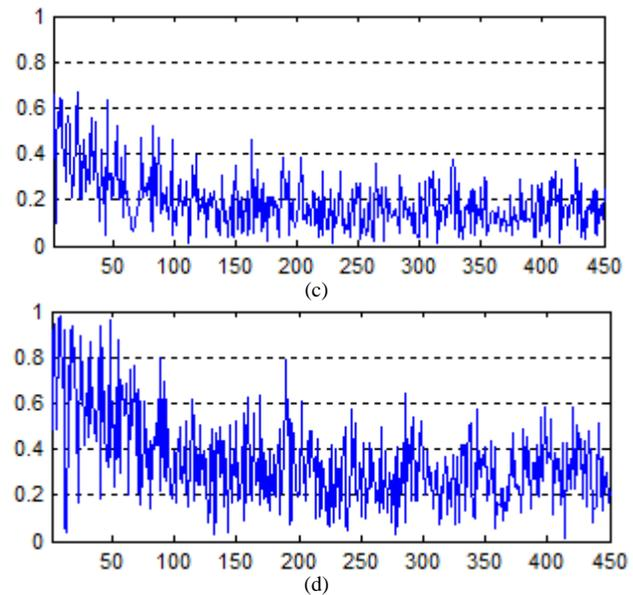
Fig. 13:  $\Delta\sigma$  versus frequency of each mode (mode order in absisse) for (a) Cavity\_1, (b) Cavity\_2, (c) Cavity\_3, (d) Cavity\_4.
