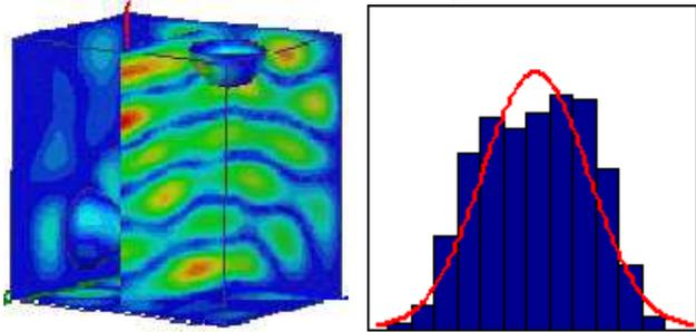
Fig. 6: Electric field amplitude and associated distribution of  $E_x$  component at 913MHz (174<sup>th</sup> mode) for Cavity\_2 (KS=1)
