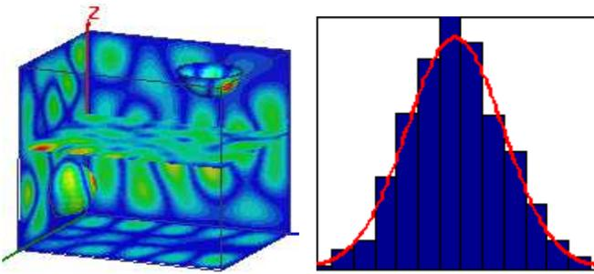
Fig. 5: Electric field amplitude and associated distribution of  $E_x$  component at 995MHz (228<sup>th</sup> mode) for Cavity\_2 (KS=0)
