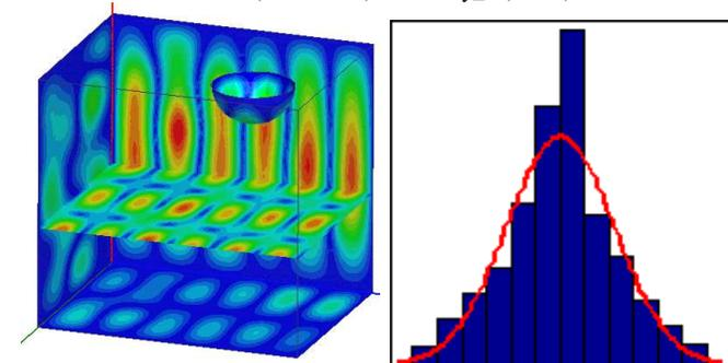
Fig. 4: Electric field amplitude and associated distribution of  $E_x$  component at 994MHz (230<sup>th</sup> mode) for Cavity\_1 (KS=1)
