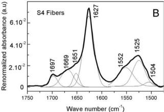
**Fig. 3.** Decomposed FT–IR spectrum of S4 peptides (A) and S4 fibers (B) in the amide I–II zone (bold line: experimental curve; fine lines: decomposition into Gaussian peaks and sum of the Gaussian peaks).
