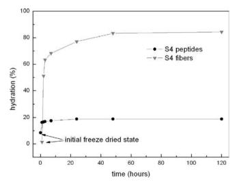
Fig. 5. Water sorption of S4 peptides and S4 fibers under 53% RH at 25 °C.
