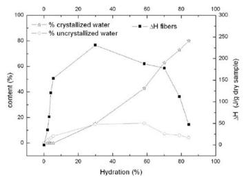
**Fig. 8.** Amounts of crystallized and uncrystallized water in S4 hydrated fibers and enthalpy of the second endothermic peak as a function of the total hydration of S4 fibers computed from Fig. 7.
