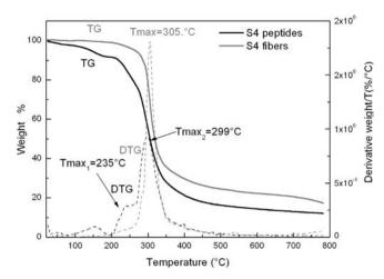
**Fig. 4.** TGA thermograms (TG) and temperature derivative (DTG) thermograms of freeze-dried S4 peptides and freeze-dried S4 fibers.
