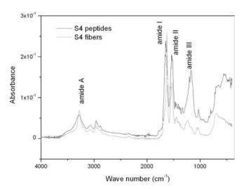
Fig. 2. FT-IR/ATR spectra of freeze-dried S4 peptides and S4 fibers.
