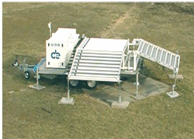
Figure 2a Bamako UHF PCL 1300 Wind profiler radar
