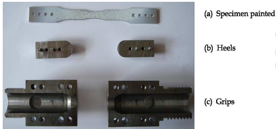
Figure 2: Grip system used in the dynamic tensile test.
