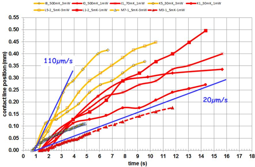
Figure 7: Preliminary results of the contact line moving for a representative set of heat pulses observed in the DOC during the ALI5-Seq7 run. *Blue lines*: preliminary estimations of the maximum and minimum speeds, respectively.
