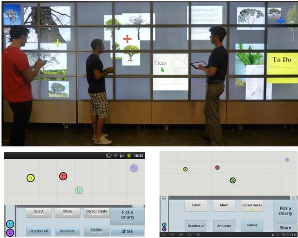
**Figure 3. Object selection and grouping with three users.** The interface running on a *phone* (left, middle user) and on a *tablet* (right, right user). Six state button widgets have been added by the application. The "Cursor Inside" action (device on the right) is attached to the active green puck, and acts as a mouse cursor confined inside a window.
