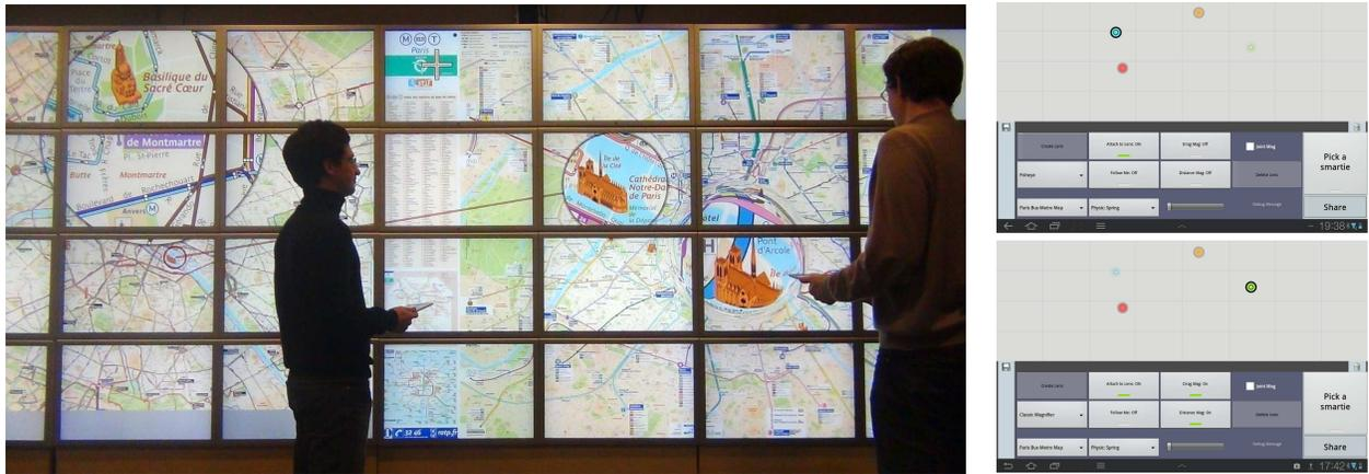
**Figure 5.** Left: Multiple Lenses, starting from the left a magnification lens, a DragMag and a fisheye. Right: the two mobile client interfaces running on tablets. The four pucks are attached respectively to a magnification lens (left of wall), the anchor and lens of a DragMag (middle) and a fisheye (right). The active puck is the blue for the device on top, and green for the bottom. The described widgets added by the application are seen on the widget area.
