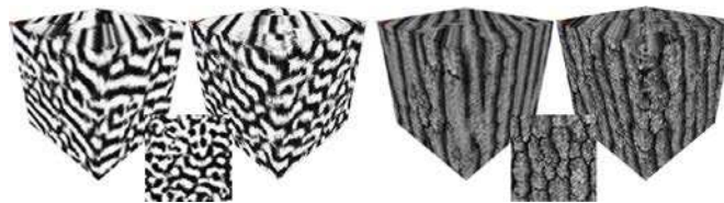
Figure 7 – Volumetric results obtained with different relaxation algorithms over the ML_H2b heuristic: each example contains in the middle the 2D sample texture, on the left the result obtained using the deterministic relaxation algorithm and on the right, the result corresponding to the simulated annealing based synthesis process.
