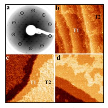
FIG. 2. (Color online) (a) LEED pattern (inverted contrast for clarity) recorded at 80 eV on the surface annealed to 1103 K for 1 h. (b)–(d)  $100 \times 100$  nm<sup>2</sup> STM images showing the terrace and step morphology for different annealing time and temperatures: (b) T =1115 K for t=1 h, (c) T=1115 K for t=2 h, and (d) T=1165 K for t=1 h. The two types of terminations are labeled T1 and T2 on (b) and (c).
