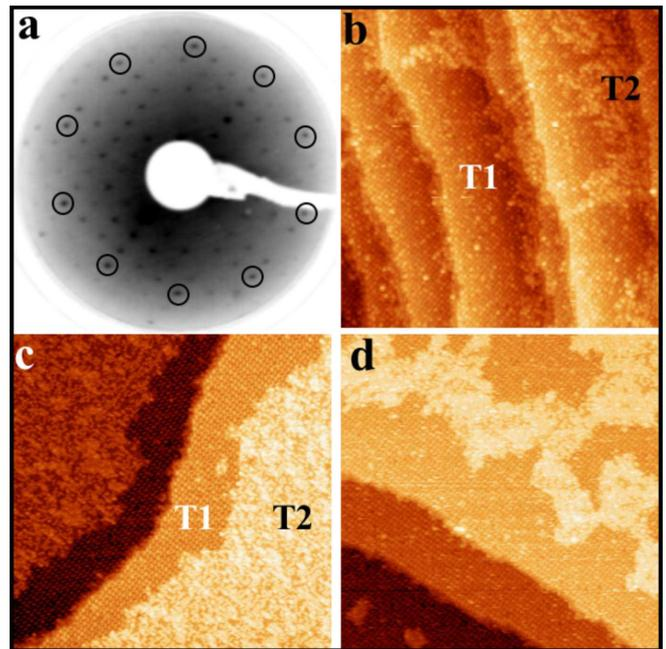
FIG. 2. (Color online) (a) LEED pattern (inverted contrast for clarity) recorded at 80 eV on the surface annealed to 1103 K for 1 h. (b)–(d)  $100 \times 100 \text{ nm}^2$  STM images showing the terrace and step morphology for different annealing time and temperatures: (b)  $T = 1115 \text{ K}$  for  $t = 1 \text{ h}$ , (c)  $T = 1115 \text{ K}$  for  $t = 2 \text{ h}$ , and (d)  $T = 1165 \text{ K}$  for  $t = 1 \text{ h}$ . The two types of terminations are labeled T1 and T2 on (b) and (c).
