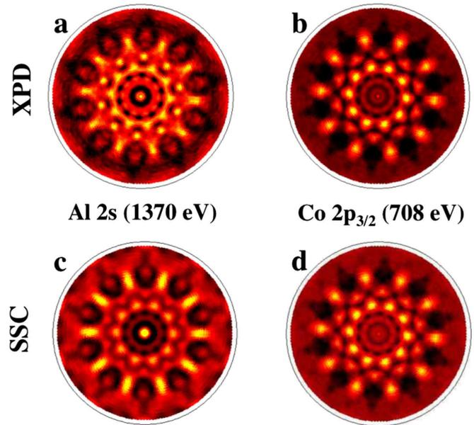
FIG. 5. (Color online) Experimental XPD patterns of (a) Al  $2s$  and (b) Co  $2p_{3/2}$  core levels measured on the  $\text{Al}_{13}\text{Co}_4$  (100) surface with an Al  $K_{\alpha}$  (1486.7 eV) x-ray source. (c) and (d) Single scattering cluster simulations for Al  $2s$  ( $E_{kin}=1370$  eV) and (d) Co  $2p_{3/2}$  ( $E_{kin}=708$  eV) emission based on a cluster of 3016 atoms derived from the bulk model (Ref. 12) described in Fig. 1.
