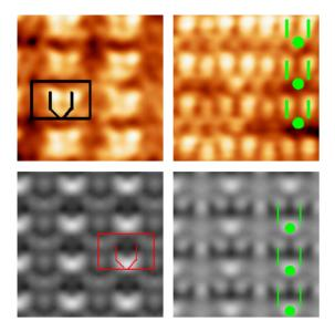
FIG. 11. (Color online) Comparison between experimental STM images recorded for the S-type terrace (top row) and simulated STM images for the PP model (bottom row). The left column corresponds to  $V_{bias}$ =-0.5 V, the right column to  $V_{bias}$ =+0.5 V.
