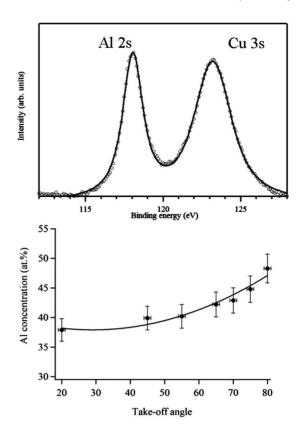
FIG. 2. Top: XPS spectra of the Cu 3s and Al 2s core levels of the  $\gamma$ -Al<sub>4</sub>Cu<sub>9</sub> (110) surface recorded at a take-off angle of  $45^\circ$ . Bottom: calculated Al content (in at. %) as a function of the take-off angle of the photoelectrons. Solid line is a fit of the experimental data points.
