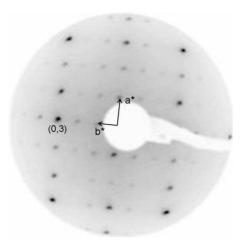
FIG. 1. LEED pattern of the  $\gamma$ -Al<sub>4</sub>Cu<sub>9</sub> (110) surface recorded at a primary beam energy of 60 eV.
