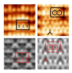
FIG. 12. (Color online) Comparison between experimental STM images recorded for the L-type terrace (top row) and simulated STM images for the PF model (bottom row). The left column corresponds to  $V_{bias}$ =-0.5 V, the right column to  $V_{bias}$ =+0.5 V.
