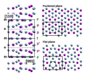
FIG. 6. (Color online) Left: atomic structure of γ-Al<sub>4</sub>Cu<sub>9</sub> projected along the [110] direction. The letters m and n indicate the positions of mirrors planes. Right: atomic structures of puckered and flat planes. Light gray (blue) and dark gray (pink) dots are for Cu and Al atoms, respectively.
