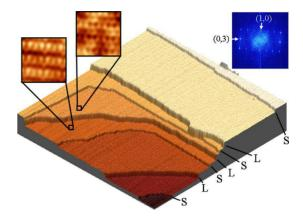
FIG. 4. (Color online) Three-dimensional view of the  $\gamma$ -Al<sub>4</sub>Cu<sub>9</sub> (110) surface (STM, 200×200 nm²,  $I_t$ =0.2 nA, and  $V_b$ =+1.4 V) showing alternating S (2.2±0.1 Å) and L (4.4±0.1 Å) steps. Insets show the two different types of STM contrast observed on S and L terraces (4×4 nm²,  $I_t$ =0.3 nA, and  $V_b$ =+0.5 V) and the FFT of an STM image of  $\gamma$ -Al<sub>4</sub>Cu<sub>9</sub> (110) surface.
