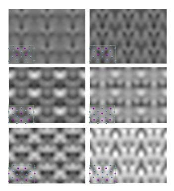
FIG. 9. (Color online) STM images simulated from the three bulk-terminated slabs: F (top), PP (middle), and PF (bottom). The images are plotted for a constant tip-surface distance ( $\approx 3\,$  Å) using two different bias voltages:  $-0.5\,$  V (left) and  $+0.5\,$  V (right). A unit cell is superimposed on the simulated images (the dark circles represent the aluminum atoms whereas the gray circles represent the copper atoms).
