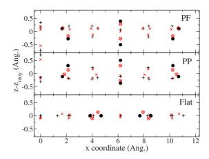
FIG. 8. (Color online) Atomic relaxation of the outermost atomic planes with respect to the corresponding bulk planes for the three types of terminations PP, PF, and F of the (110)  $\gamma$ -Al<sub>4</sub>Cu<sub>9</sub> surface. The filled circles (respectively, plus features) are Al atoms (respectively, Cu atoms) in the bulk plane, the crossed circles (respectively, times features) are Al atoms (respectively, Cu atoms) in the surface planes.
