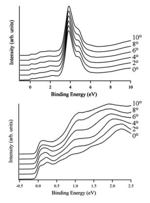
FIG. 3. Top: valence-band spectra of the  $\gamma$ -Al<sub>4</sub>Cu<sub>9</sub> (110) surface recorded at different take-off angle. The main peak at 4 eV corresponds to Cu d states. Bottom: near  $E_F$  spectra showing dispersive features.
