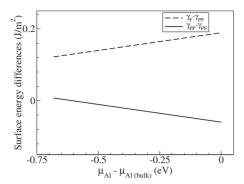
FIG. 7. Variation with the chemical potential of Al atoms of the surface energy of F and PP surface terminations referred to the PF termination.
