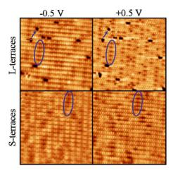
FIG. 5. (Color online) Images ( $15 \times 15 \text{ nm}^2$ ,  $I_t$ =0.3 nA) illustrating the bias dependency of the STM contrast for L and S terraces. Surface vacancies (arrows) and possible chemical inhomogeneities (circles) are highlighted.
