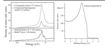
FIG. 4. Left: Electronic DOS of the surface and subsurface layers of Al<sub>13</sub>Fe<sub>4</sub>. Right: Ultraviolet photoelectron spectroscopy valence-band spectrum of the clean surface.
