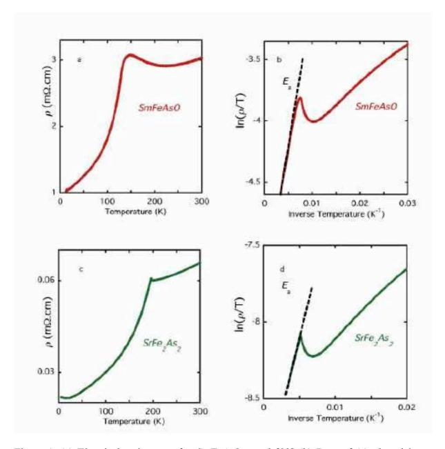
Figure 1. (a) Electrical resistance of a *SmFeAsO* sample[32] (b) Data of (a) plotted in an Arrhenius plot (logarithm of resistivity/temperature versus inverse temperature) in order to determine the activation energy  $E_a$  due to small polaron transport (c) Electrical resistivity of a *SrFe*<sub>2</sub>*As*<sub>2</sub> sample[33] (d) Same as (c) for the *SrFe*<sub>2</sub>*As*<sub>2</sub> sample.
