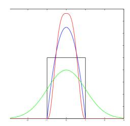
FIGURE 1. Example of kernels. They are normalized in order to integrate to one. Black: Uniform, Blue: Epanechnikov, Red: Tricube, Green: Gaussian.
