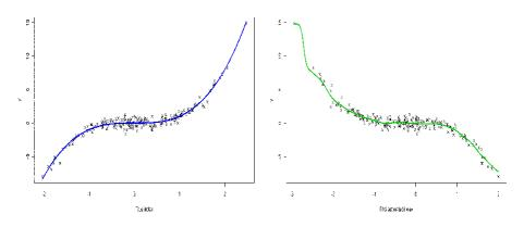
FIGURE 7. Left panel: Scatterplot of the true index versus Y,  $(X_i^t \ \beta, Y_i)$  for  $i = 1, \ldots, 200$  and true link function (blue line). Right panel: Scatterplot of the first estimated index versus Y,  $(X_i^t \ \hat{b}_1, Y_i)$  for  $i = 1, \ldots, 200$  and estimated link function (green line).
