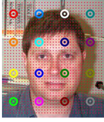
Fig. 2: Seed points. In red: the nodes of the graphs. In other colors: the seed points
