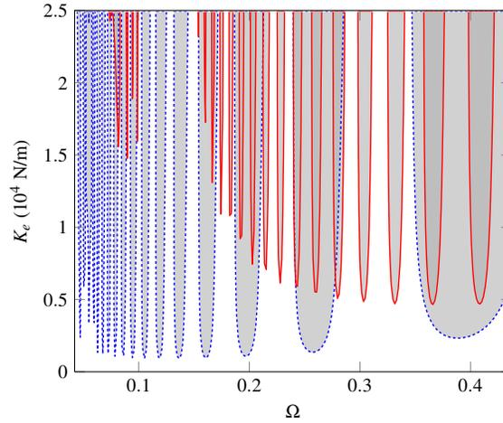
**Figure 14:** Instability lobes: bending (---) and torsion (—) modes
