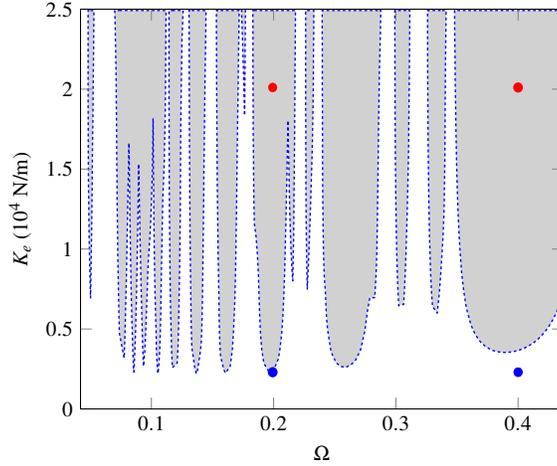
**Figure 6:** Test points: • stable domain ( $K_e = 2 \cdot 10^3$  N/m);
