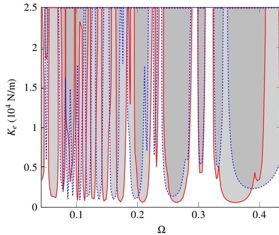
**Figure 10:** Instability lobes with (- - -) and without (—) centrifugal effects
