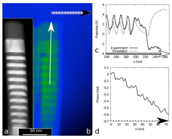
**Figure 2.** (a) HAADF STEM image of a GaN/AlN NW heterostructure. (b) Phase image of the same NW. (c) Potential profile obtained from the phase along the vertical white arrow compared with two simulated profiles one including a surface charge density of  $-2x10^{13}$  electron charges cm<sup>-2</sup> and one without surface charges. (d) Phase profile in the vacuum obtained along the horizontal black dotted arrow.
