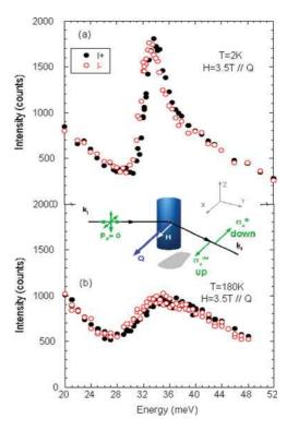
FIG. 2. (Color online) (a) Energy scans taken at Q = (-4.5,0,0.5) with *half*-polarized neutrons at T = 2 K and under a magnetic field of 3.5 T parallel to Q. Solid and empty circles correspond to two different states of polarization. (b) The same as (a) but at T = 180 K.
