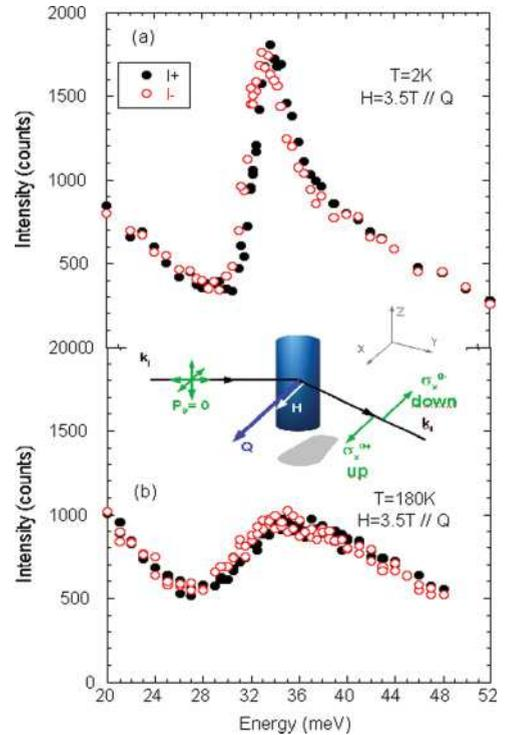
FIG. 2. (Color online) (a) Energy scans taken at  $Q = (-4.5, 0, 0.5)$  with *half*-polarized neutrons at  $T = 2$  K and under a magnetic field of 3.5 T parallel to  $Q$ . Solid and empty circles correspond to two different states of polarization. (b) The same as (a) but at  $T = 180$  K.
