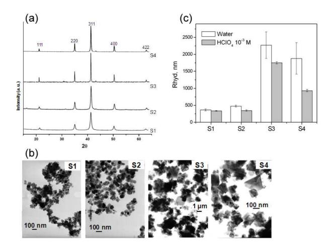
**Figure 1:** XRD (a) and TEM (b) images of the four used magnetite samples; (c) Hydrodynamic radii (R<sub>hyd</sub>) of the magnetite particles/aggregates, measured by Dynamic Light Scattering in pure water and in 1 mM HClO<sub>4</sub>. Error bars represent 95% confidence intervals.
