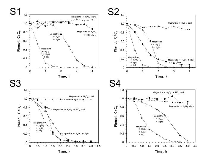
**Figure 2.** Time trend of phenol (initial concentration 0.1 mM, pH 3 by  $HClO_4$ ) under photo-Fenton conditions (phenol +  $H_2O_2$  + magnetite S1-S4 + UVA) and in blank runs. When relevant, other conditions were as follows: 1 mM  $H_2O_2$ , 0.2 g  $L^{-1}$  magnetite loading, 50  $\mu$ M added HQ.
