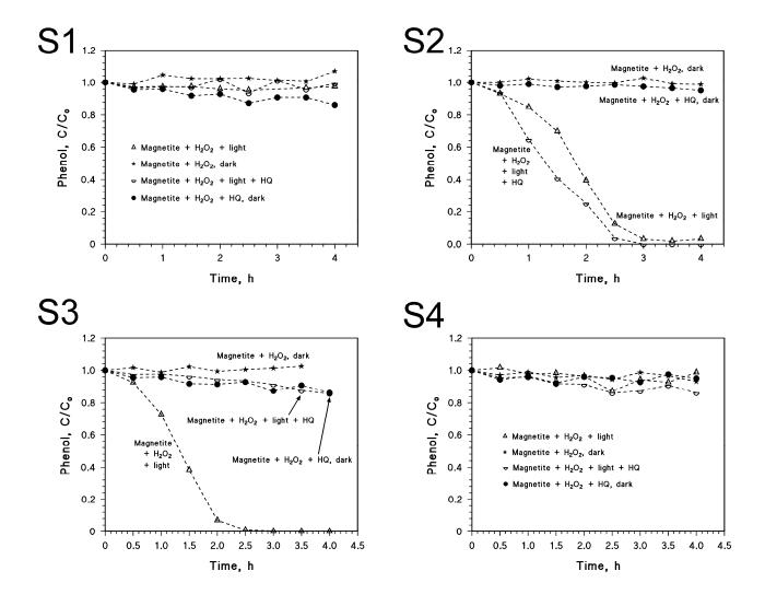
**Figure 4.** Time trend of phenol (initial concentration 0.1 mM, pH 6) under photo-Fenton conditions (phenol +  $H_2O_2$  + magnetite S1-S4 + UVA) and in blank runs. When relevant, other conditions were as follows: 1 mM  $H_2O_2$ , 0.2 g  $L^{-1}$  magnetite loading, 50  $\mu$ M added HQ.
