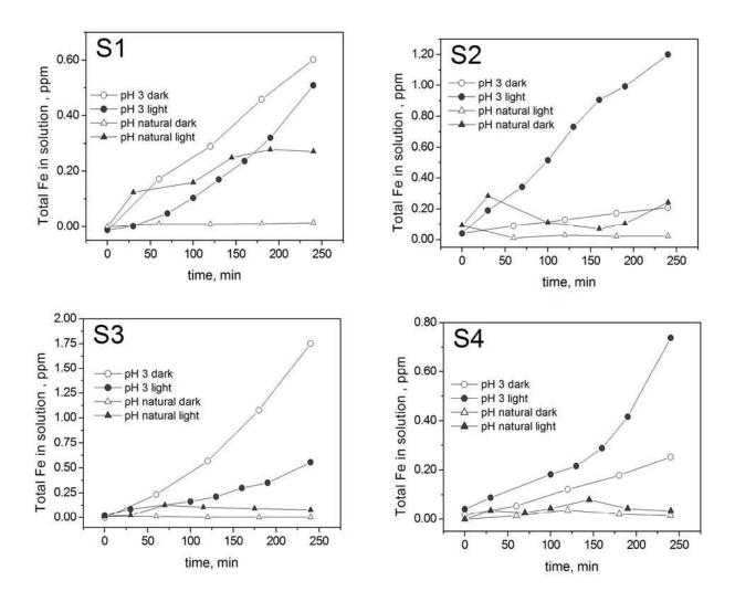
**Figure 3.** Total iron released in solution, both in the dark (open symbols) and under irradiation (solid symbols), at pH 3 by HClO<sub>4</sub> (circles) and at pH 6 (natural pH, triangles), in the presence of the studied magnetite samples. Conditions were as follows: initial phenol concentration 0.1 mM, 1 mM H<sub>2</sub>O<sub>2</sub>, 0.2 g L<sup>-1</sup> magnetite loading.
