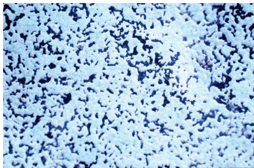
Figure 1. Macroscopic view of black spots surrounded by green pale corrosion products, porous and unprotected.
