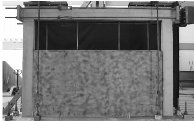
45 Fig. 8 Single bay partially infilled frame (PF)
