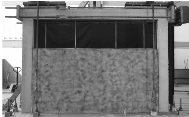
45 Fig. 8 Single bay partially infilled frame (PF)
