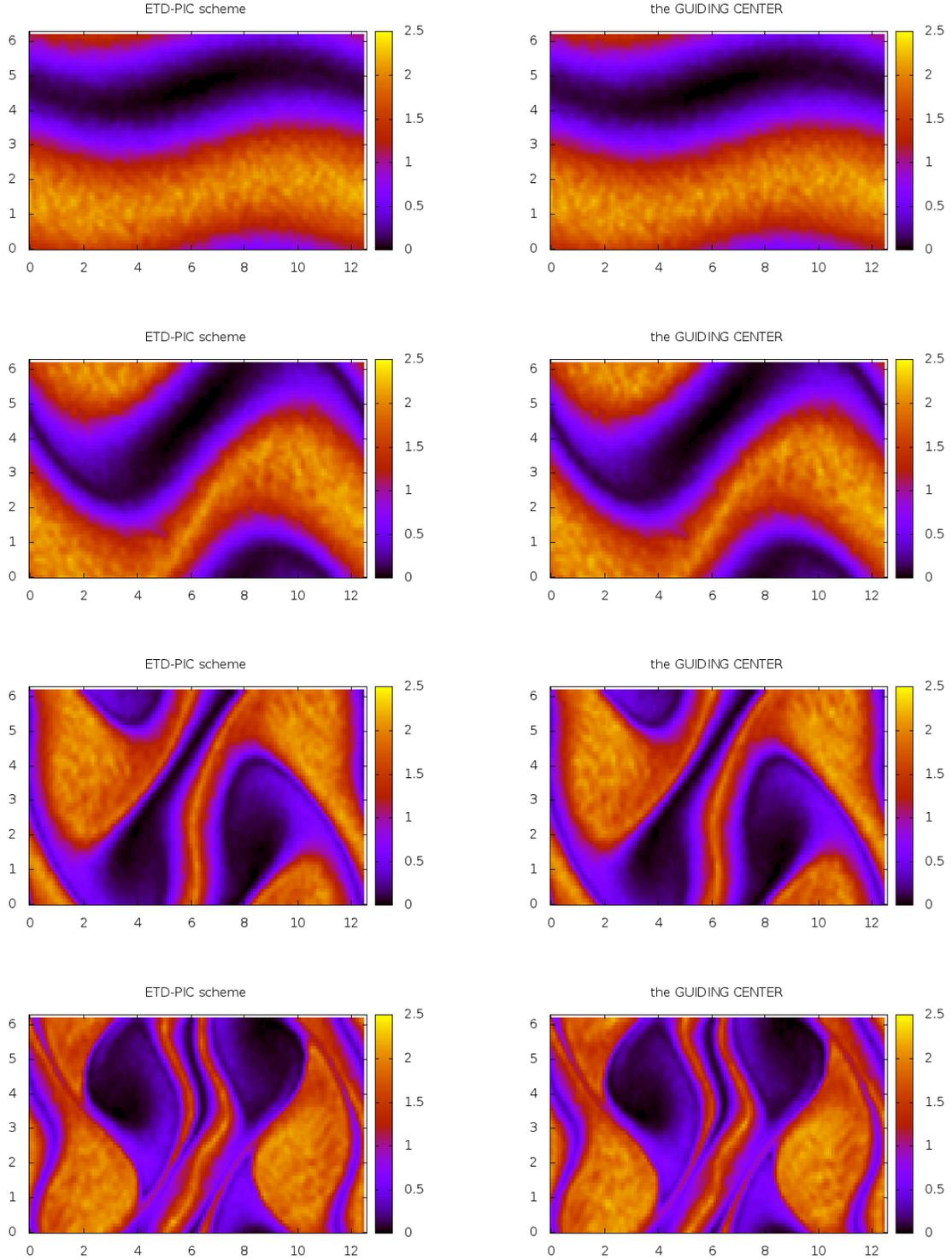
Figure 8: Simulations of  $\rho_g^\varepsilon$  with the ETD-PIC method when  $\varepsilon = 0.005$  (left) and of the Guiding Center distribution function (right). From top to bottom we represent the densities' contours at times  $t = 5$ ,  $t = 10$ ,  $t = 15$ , and  $t = 20$ . The time step is  $\Delta t = 0.01$  (The number of fast periods in  $\Delta t$  is  $N = 63$ ).
