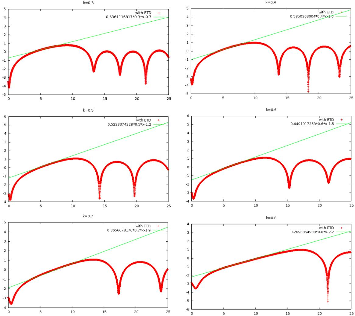
Figure 10: In red, the evolution in time of the logarithm of the absolute value of the (1, 1) Fourier coefficient of  $\psi^\varepsilon$ . In green, the growth rate obtained through the eigenvalue equation (see Table 4). Simulations with fixed  $\Delta t = \varepsilon = 0.005$  and several values of  $k$  between 0.3 and 0.8 in the definition of the initial condition in (5.31)
