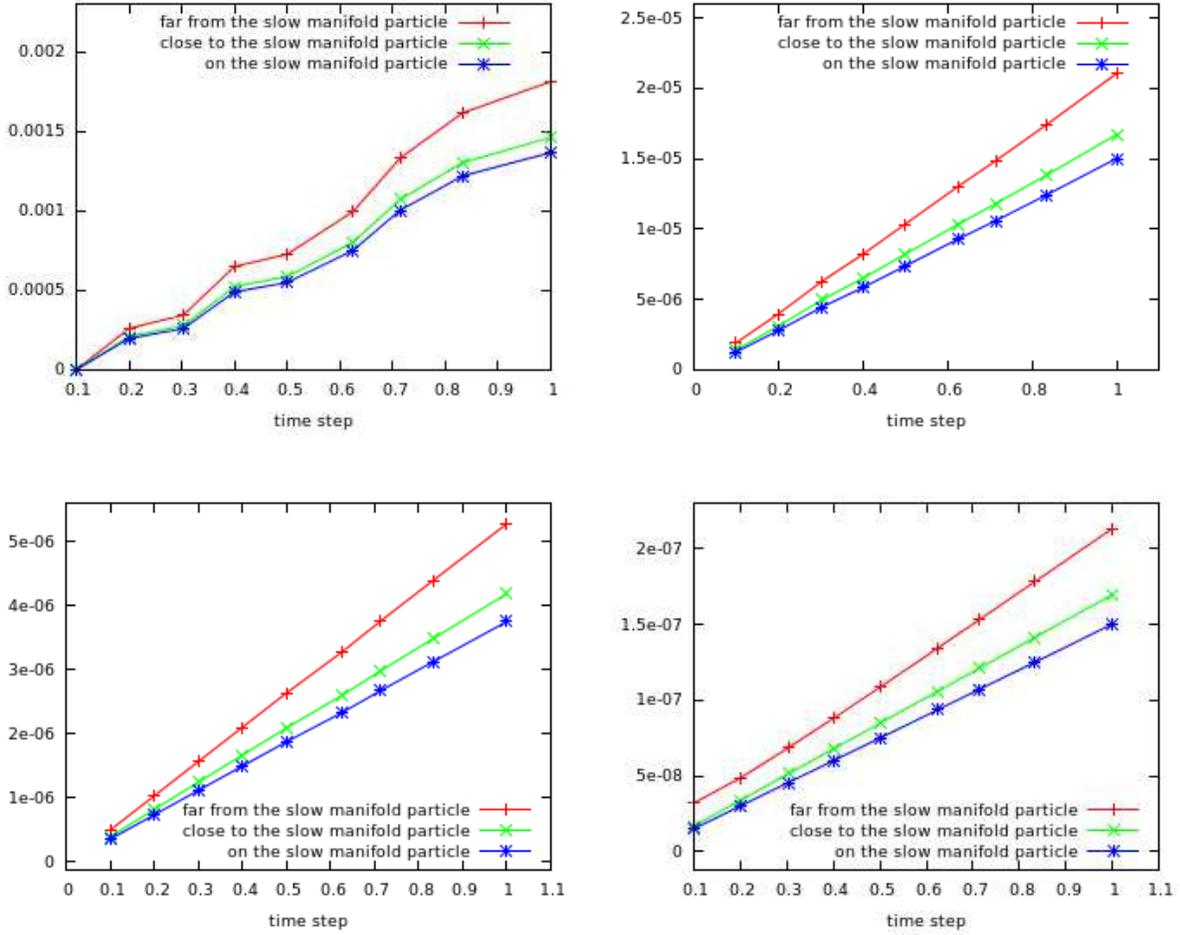
Figure 3: Global Euclidean errors of the ETD-PIC method at time 10 for four values of  $\varepsilon$  (on the top:  $\varepsilon = 0.01$  (left) and  $\varepsilon = 0.001$  (right); on the bottom:  $\varepsilon = 0.0005$  (left) and  $\varepsilon = 0.0001$  (right)), obtained with three initial conditions differently positioned with regard to the slow manifold  $\mathcal{D}_2$
