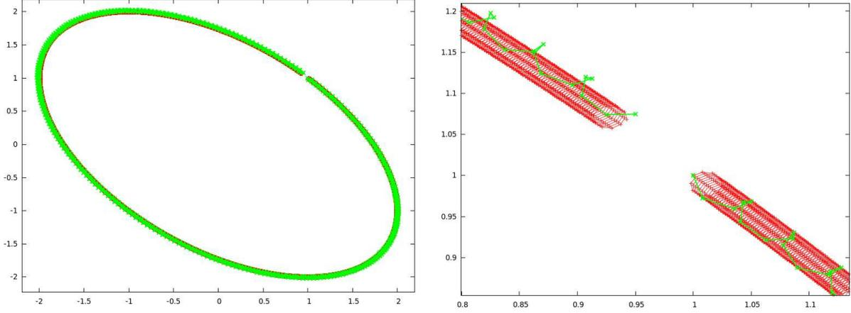
Figure 2: The linear case in Section 5.1 with  $\varepsilon = 0.01$  and the initial condition  $(1, 1, 1, 1)$ : the position's evolution in time until  $t = 360$ ; the entire trajectory (left) and a zoom at the beginning of the dynamics (right); In green the result of the ETD scheme using a time step  $\Delta t = 30\varepsilon$  and in red the analytic solution given in formulas (5.1)
