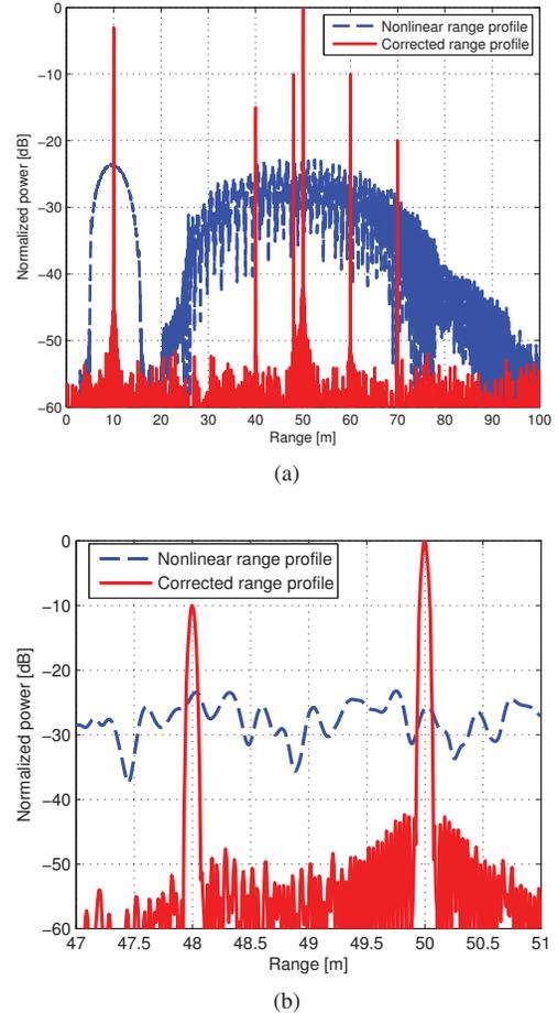
**Fig. 2:** Range profiles simulation results: (a) 0-100m range, (b) detailed 47-51m range. In the nonlinear range profile five targets are completely indistinguishable. The corrected range profile leads to a resolution near the theoretical limit and improves the signal to noise ratio.
