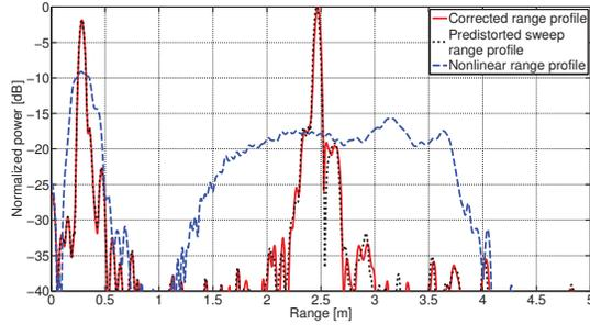
**Fig. 3:** Experimental range profiles for two delay lines. The range profile obtained with the nonlinearity correction algorithm is compared with the predistorted sweep range profile and with the nonlinear range profile corresponding to the linear voltage sweep.
