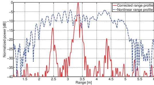
**Fig. 4:** Experimental range profiles for a scene containing two metal bars and one highly reflective metal disc. On the corrected range profile the three targets are clearly separated, while in the nonlinear range profile the scatterers can't be distinguished.
