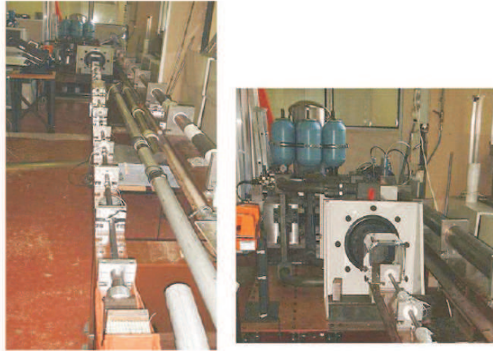
Fig. 40a View of the slow bar rig Fig. 40b Hydraulic actuator
