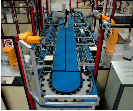
Fig 11. The pallet transfer system “SISTRE”
