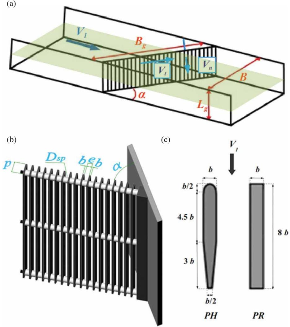
Figure 1 Representation of the angled trashrack in the channel (a) and details on the initial segment of the trashrack (b) with the two bar shapes tested (c). The green plane on the overall view represents the position of the laser sheet in PIV measurements
