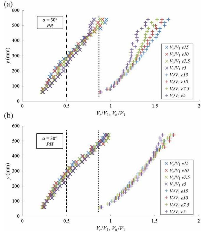
Figure 6 Comparison of  $V_t/V_1$  and  $V_n/V_1$  profiles along the angled rack ( $\alpha = 30^\circ$ ) for different bar spacings  $e$  and bar shapes. The dashed and dotted vertical lines show the theoretical values for  $V_n/V_1$  and  $V_t/V_1$  respectively, calculated by geometrical projection
