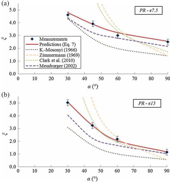
Figure 3 Comparison of measured head-loss coefficients and coefficients predicted by the quoted equations. Bars are rectangular and  $e = 7.5$  mm, i.e.  $e/b = 1.5$  (a) and  $e = 15$  mm, i.e.  $e/b = 3$  (b)
