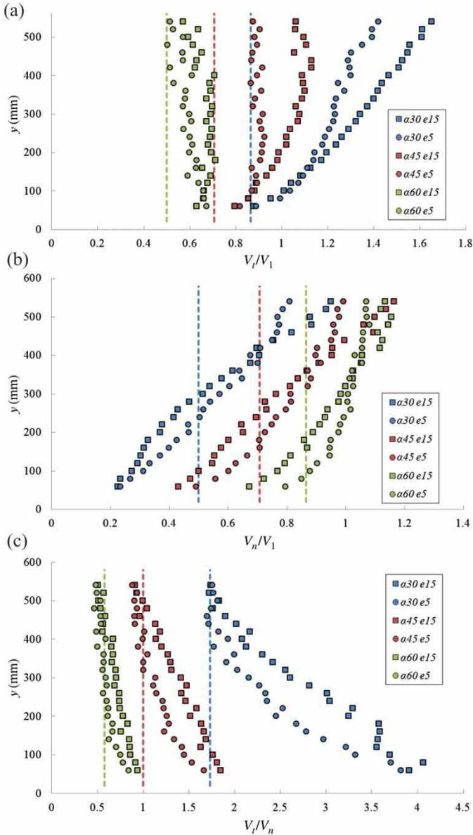
Figure 7 Comparison of  $V_t/V_1$  (a),  $V_n/V_1$  (b) and  $V_t/V_n$  (c) profiles for three PR trashrack angles (30, 45 and 60°, respectively the blue, red and green marks) and two bar spacings (5 and 15 mm, respectively, the round and square marks). Dashed lines represent theoretical values obtained by geometrical projection
