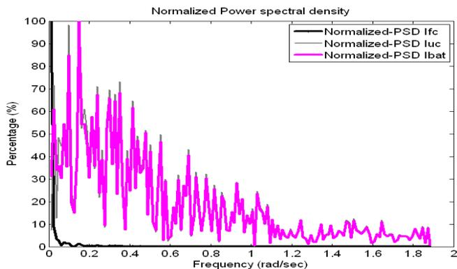
Fig. 9. Normalized power spectrum of the sources' currents corresponding to IFSTAR load current profile by using LQR approach.
