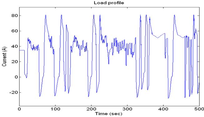
Fig. 6. IFSTTAR load current profile used in simulation.
