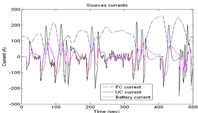
Fig. 11. Sources' currents according to  $H_\infty$  approach.
