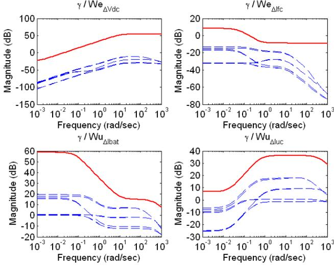
Fig. 5. Weighting function used to confine frequency ranges of battery and ultracapacitor current variations within imposed frequency domains.
