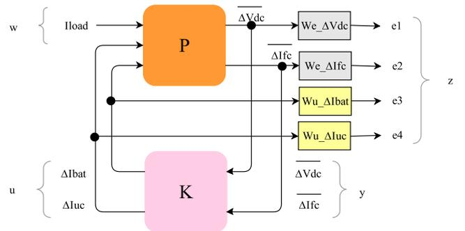
Fig. 4.  $H_\infty$  Robust control design block diagram.
