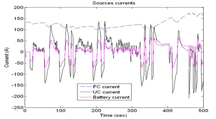
Fig. 7. Sources' currents according to LQR approach.
